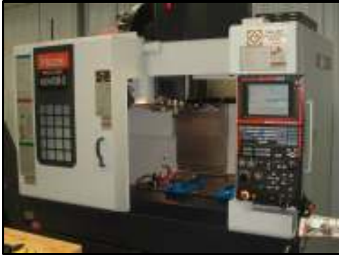
Mazak vertical machining center 16" x 32" travels w/30 position tool changer
