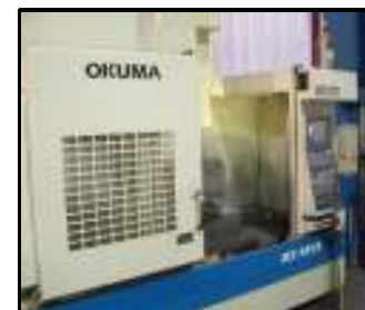
Okuma vertical machining center 20" x 40" travels w/20-position tool changer
