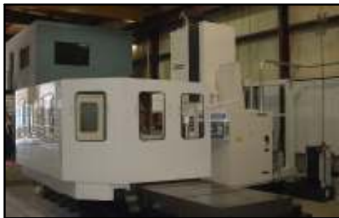
Toshiba HMC CNC BP-150.R22 160" x 120" x 60" w/360° rotary table w/60 pos. automatic tool changer
